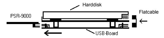
Important: Take care that the raisings of the metal plate are in direction of the hard disk, this is to prevent a short circuit between the hard disk and the metal plate.
