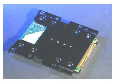
Now put on the holes that used for fasten the hard disk the four plastic separation rings. Put on the USB-Interface board on it and mount all together with the four attached screws.
